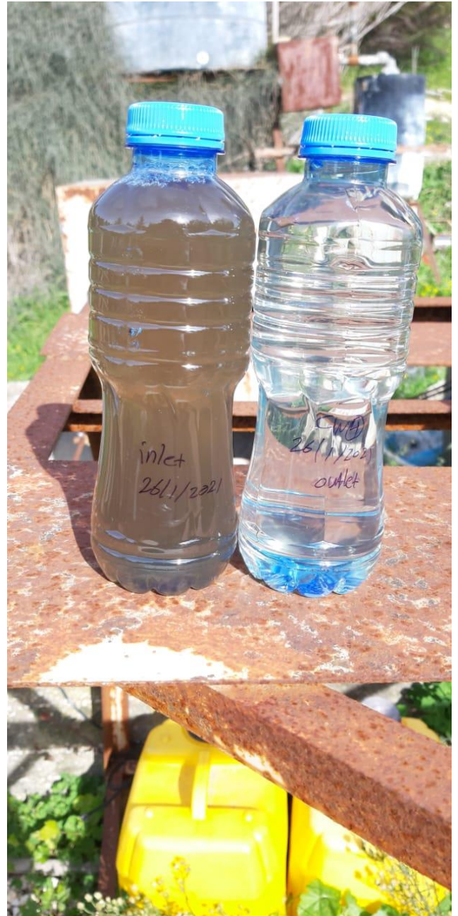
water inlet and outlet of constructed wetlands
